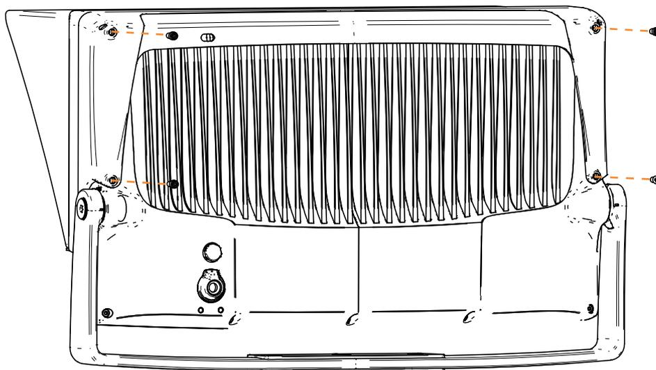
NOTE: Do not remove any screws from the luminaire body to secure the accessory holder.
