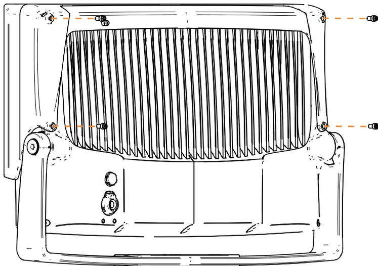
NOTE: Do not remove any screws from the luminaire body to secure the accessory holder.
