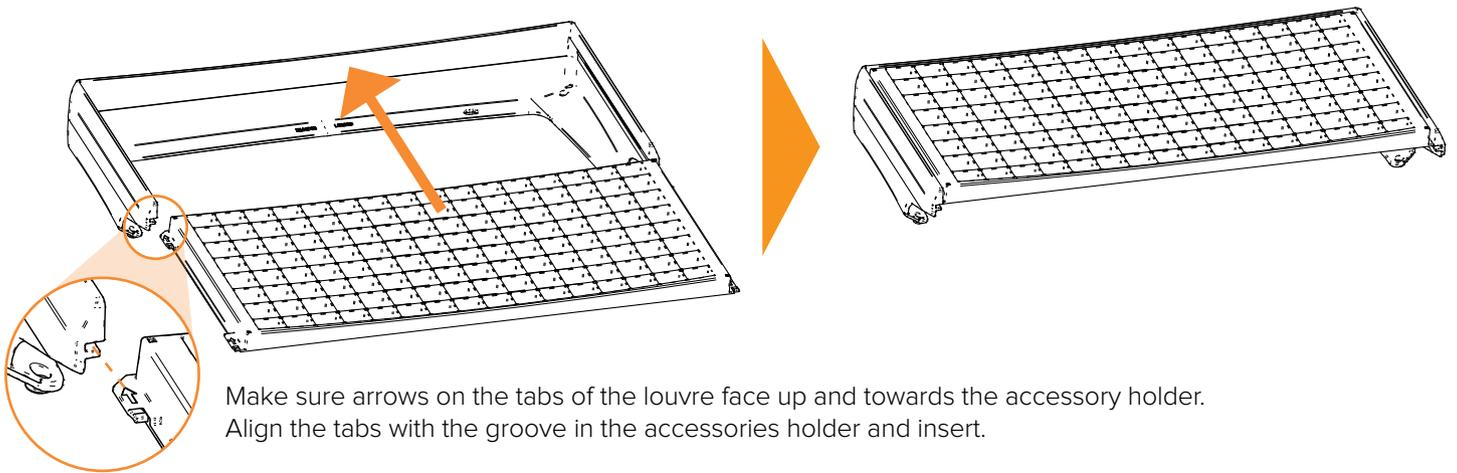
Slip the accessory holder & louvre assembly over the luminaire
