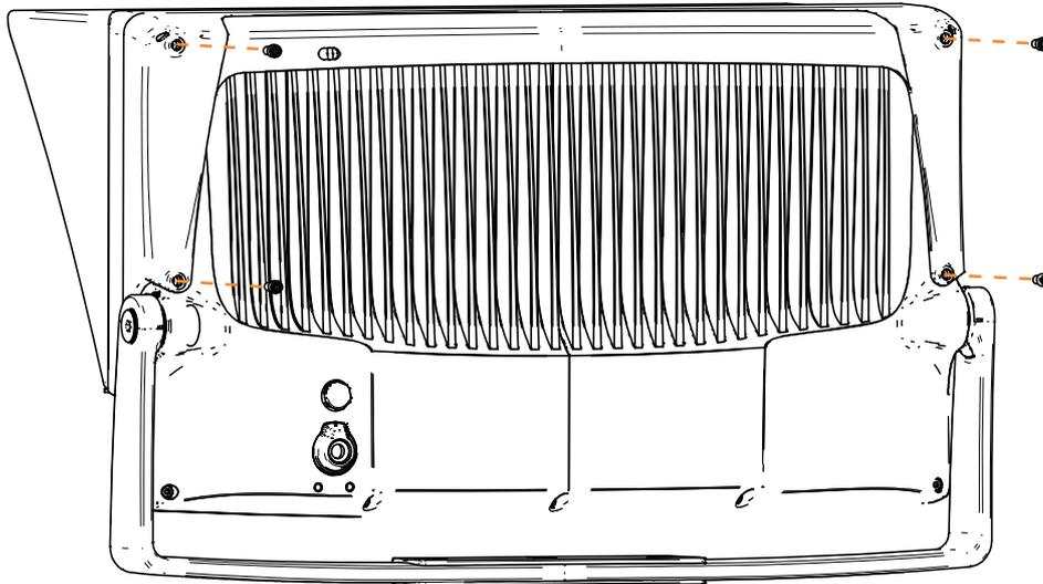
NOTE: Do not remove any screws from the luminaire body to secure the accessory holder.
