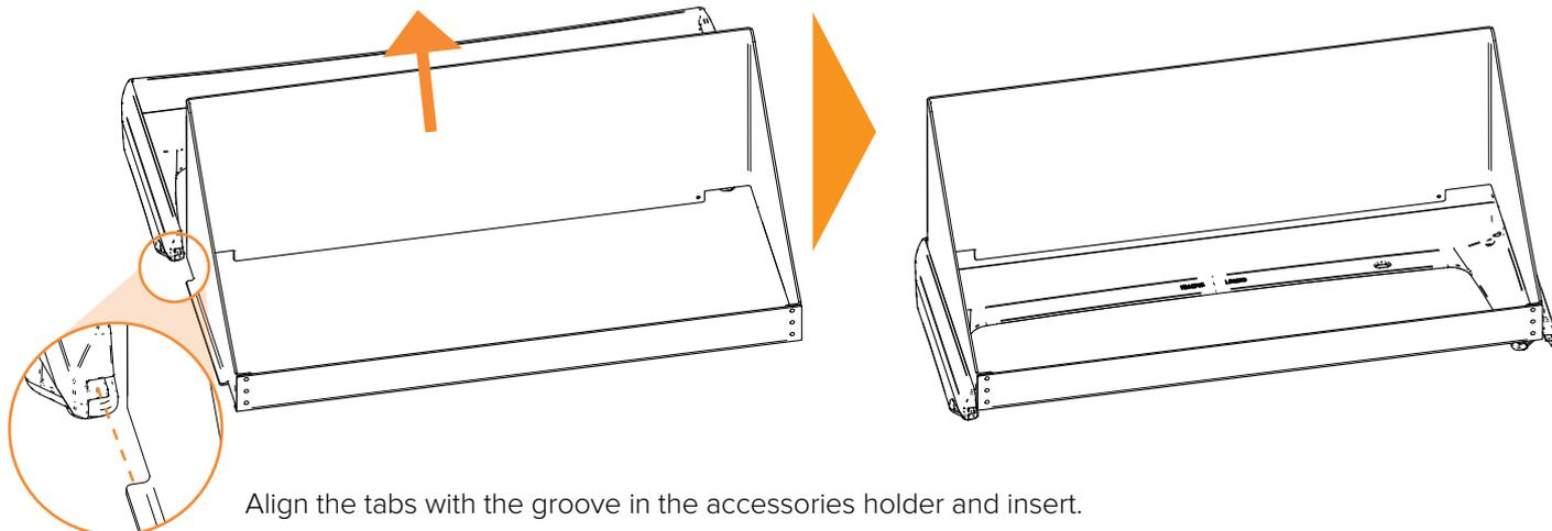
Slip the accessory holder & 45° visor assembly over the luminaire.
