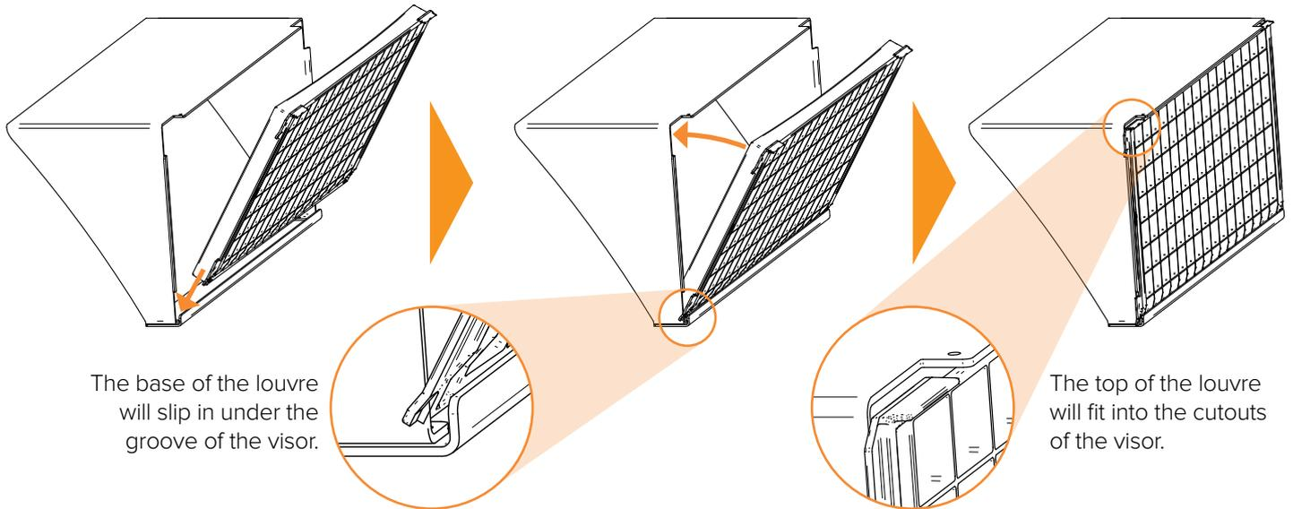
Slide 45° visor and louvre assembly into accessories holder. Make sure all the components have the right orientation and alignment as shown below.
