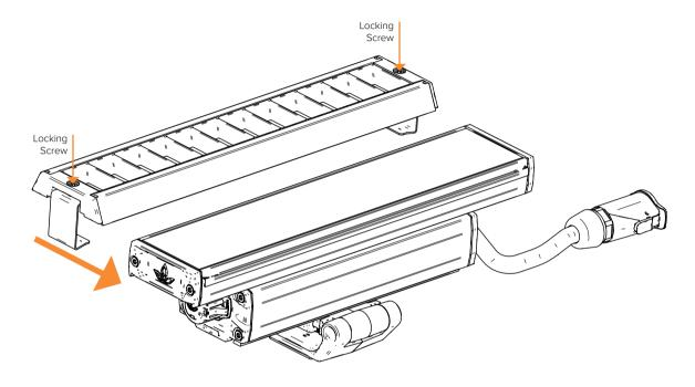
Secure the louvre tightening the locking screws.
