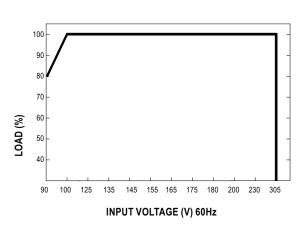
X De-rating is needed under low input voltage.
