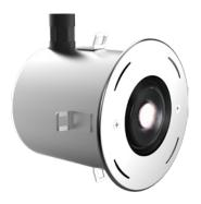
The Nero NE1 is a swimming pool rated luminaire constructed entirely of marine-grade 316 stainless steel. It utilizes a special alignment feature to ensure the beam of light is perpendicular to the installation surface, even if the pre-installation blockout niche is not. The use of LEDs allows for the creative introduction of color and improved energy-efficiency. This luminaire is suitable for saline waters.
