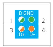
**STEP 4**Pull tab down to open terminal, then insert stranded wire.
