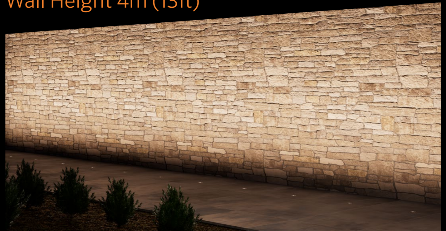
Wall height 4m (13ft) using LS332x with WP lens. Luminaire wall offset 1.4m (4.6ft). Luminaire spacing 1.8m (5.9ft).
