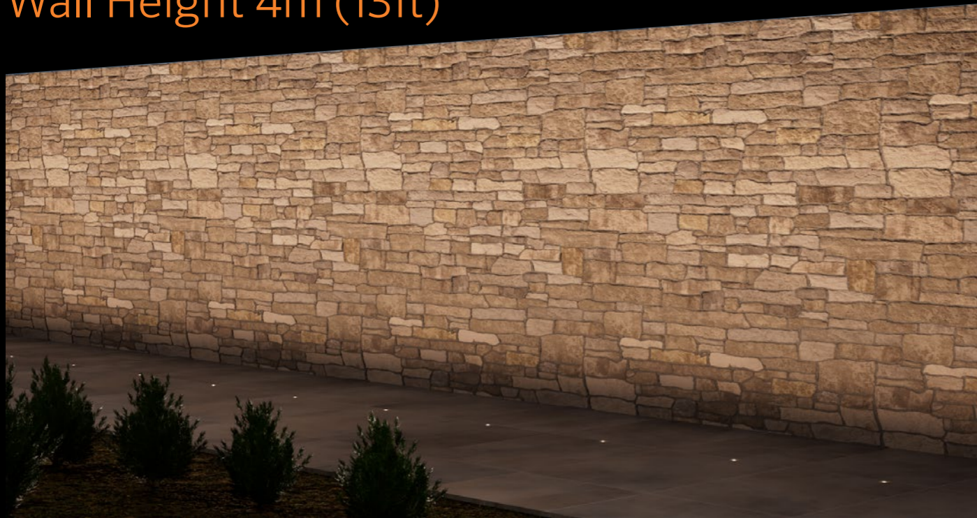
Wall height 4m (13ft) using LS332x with WS lens. Luminaire wall offset 2.0m (6.5ft). Luminaire spacing 1.9m (6.2ft).
