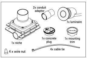
Using PVC primer and cement, glue conduit 3. adaptors supplied into required entries for 25 mm conduit. Include a draw wire within conduit. Insert concrete plug fully into niche throat. DO NOT GLUE IN.
