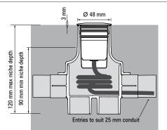
Once surface is completely installed, (including tiling, pavers or any other finishing), trim protruding niche throat flush to floor surface. Remove any burrs from inside niche throat.
