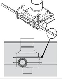
Using PVC primer and cement, glue mounting trim into niche throat. Ensure trim sits down onto and level with finished surface. Allow to fully cure as recommended by PVC cement suppliers instructions (typically 24 hours).
